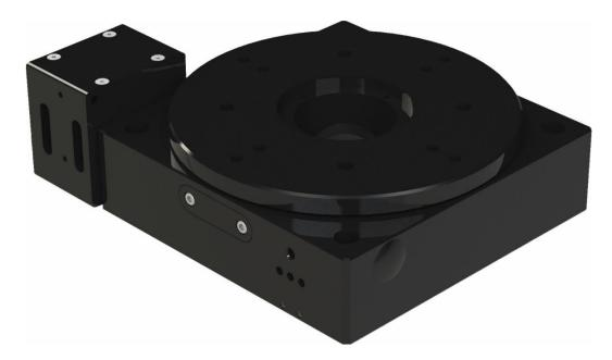
The PR150 is a worm gear driven rotary stage with a NEMA23 motor mount. Position information is by motor count, or a motor mounted rotary encoder. A high load capacity, good stiffness, and precise rotation are obtained through the use of a large, circular crossed roller bearing. Custom configurations are available such motor mounts for 5 phase stepper motors.
