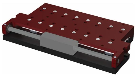
The NCR series stages are compact, low-profile stages providing high positional accuracy. Ironless servo motors provide high acceleration, making this an extremely responsive system with high position stability. Available in a variety of lengths with several force and feedback options.
