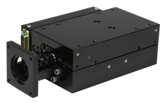
With its rigid body, center drive, and precision lapped lead screw, the HS60 stage offers superior performance for applications requiring fast step and settle performance with an open loop stepper or encoded rotary servo motor. For improved bi-directional repeatability and long-term accuracy, a non-contact, hysteresis free linear encoder is available as an option.
