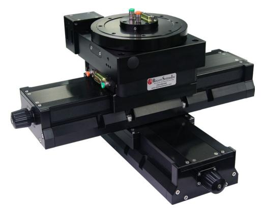
The XYO 150 stage was originally developed for a high output medical device manufacturing company. This stage assembly consists of an XY base made from our LSN series linear stages and a Theta axis made from our PR150 worm gear driven rotary stage. The Theta has an integrated slip ring which allows for cables and connections to be routed through the center aperture.
