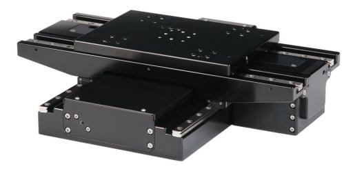
The LP150 and LP200 are low profile XY stages in a compact envelope, making them a perfect motion platform for use in desktop inspection and metrology instruments. While compact, performance is strong. Horizontal and vertical straightness of travel is  $\pm 1.0 \mu m/25 mm$  and a hysteresis-free linear encoder gives positional feedback at  $0.5 \mu m$ .
