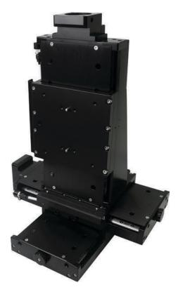
The CT101 XYZ stage was developed for a contract manufacturer that works with many medical device manufacturing companies. The specifications of having an XY with a Z axis all with 101mm of travel and high precision accuracy, repeatability, straightness, and flatness of travel made this XYZ well suited for their application. A key feature on this configuration is the NEMA23 motor mounts which allows the customer to select a motor that integrates well with their controller of choice.
