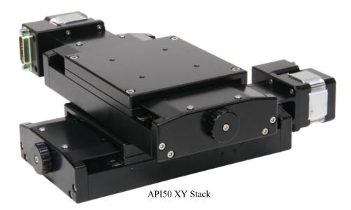
The API50 is a mid-range precision, low profile, 3mm crossed roller bearing stage with excellent stiffness and durability. The high efficiency ball screw drive uses a preloaded nut for good bidirectional repeatability without the use of a linear encoder. A NEMA17 motor mount accepts stepper, DC servo, or brushless servo motors. Optical limit and home switches provide protection with long-term reliability.
